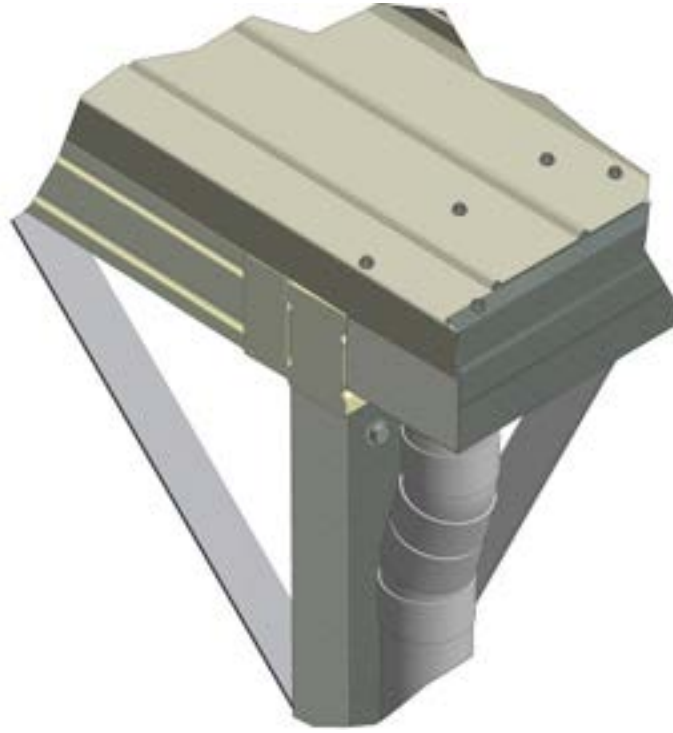
Finished Gutter Assembly - Downpipe End
