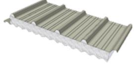
**DeltaTrimCorro-EPS-FR** is an Insulated Roof Panel System, comprising of two pre-painted, roll-formed steel skins, bonded to a fire retardant grade expanded polystyrene insulating core.
