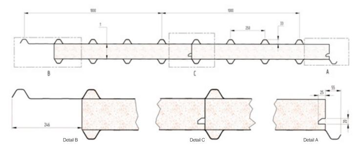
**DeltaTrimTrim-TPC** is an Insulated Roof Panel System, comprising of two pre-painted, roll-formed steel skins, bonded to a thermosetting phenolic composite insulating core.
