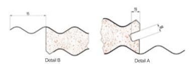
**DeltaCorroCorro-TPC** is an Insulated Roof Panel System, comprising of two pre-painted, roll-formed steel skins, bonded to a Thermosetting Phenolic Composite core.
